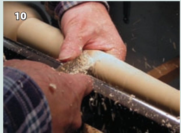
10 A shallow spindle gouge is used for final finishing. The left hand dampens vibrations and can detect errors that the eye cannot.
