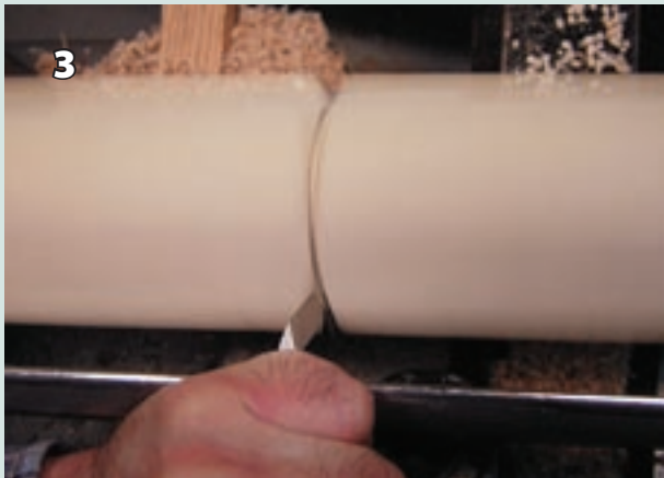
3 Making the transition cut at the node with a skew chisel.
