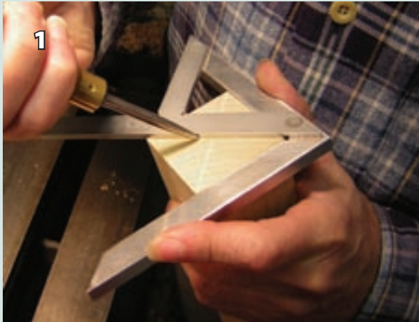
1 Using a center-square to mark diagonals. Make four lines. Squares available from Grizzly.
