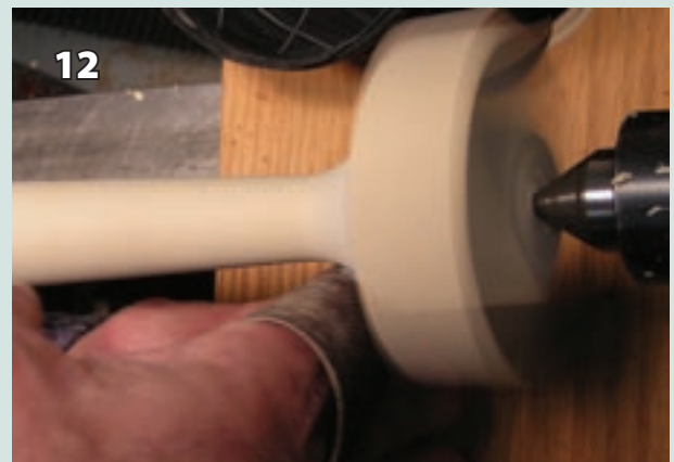
12 Light pressure and patience are required to carefully sand the intermittent part at the top of the foot.
