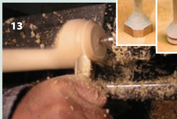
13 Use a \frac{1}{2} " spindle gouge to round the bottom of the foot. The curve begins just above the point of the toe.
