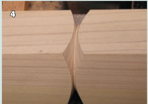
4 The transition cut completed. Notice that it is about \frac{1}{8} " deeper than the flat. The left side is the finish side.
