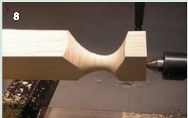
8 Top of the foot completed.
