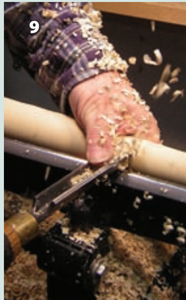
9 A \frac{3}{4} " roughing gouge is used first to taper the leg. The left hand is used to dampen workpiece vibration. The gouge is guided by the thumb.
